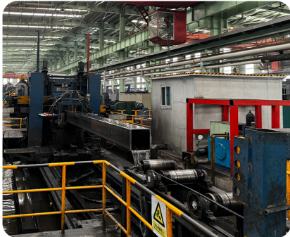
Direct Forming Line For Manufacturing Heavy-Duty Box Sections In Various Sizes And Thicknesses. With High Precision And Strength.
