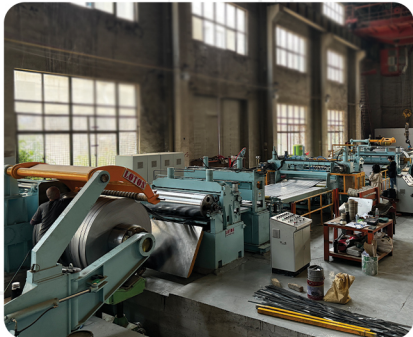
Slitting Line Designed For High-Speed And Precise Cutting Into Custom.Width Strips For Industrial Use.
