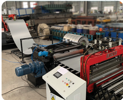
Cut-To.Length Line Delivering Precise Transverse Cuts For Converting Coils Into Uniform Sheets With Custom Lengths.
