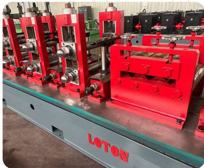
Continuous Tube Forming Line With Roll Forming Resistance Welding. Manual Die Change And Precise Quality Control.
