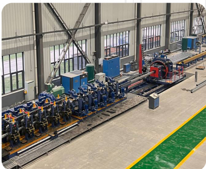
Modern Roll Forming Technology With Fast And Automatic Roll Adjustment Enables Continuous Production Of Multiple Profile Sizes Without Stopping The Line.
