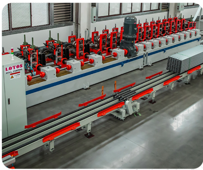
High.Speed Automatic C/U Roll Forming Line For Mass Production Of Solar Panel Structures With High Precision And Efficiency.
