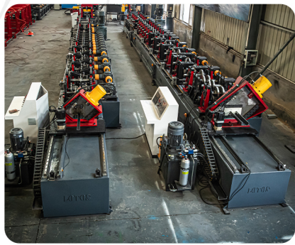
Standard.Speed CZU Roll Forming Line Designed For Reliable And Accurate Production Of Solar Panel Structures.
