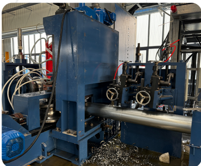
The API Pipe Production Line Utilizes Advanced Forming Technology To Continuously Produce High-Quality Steel Pipes That Meet International Standards For Oil And Gas Transmission.
